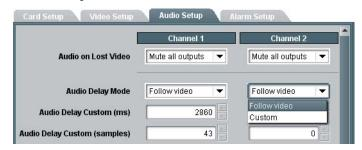
An audio delay can be specified by the user for each video input channel. Two modes are available in the **Audio Delay Mode** function. Select from:
